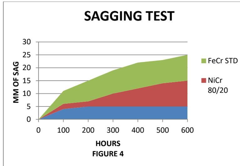
The tests were performed on 4 mm diameter rods in a horizontal position, supported at 200 mm intervals, and exposed to 1200°C. The results are shown in millimeters of sag plotted on the vertical axis against time on the horizontal axis. As indicated, the PM grade material is superior to its parent alloy.
