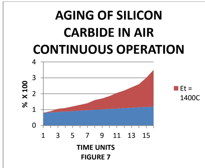
The diagram shows that an element operating at 1000°C has increased its resistance by a factor 1.5 times over fifteen (15) time units. The same element operating at 1400°C has increased its resistance by over four (4) times during the same fifteen (15) time units and has reached the end of its life.
